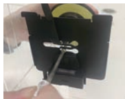
4. Align the camera plug with the mounting plate.
