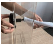
2. Place the cable through the door, from the outside in. [Note- if the door is thick, please wrap the cable in paper avoid breaking it].
