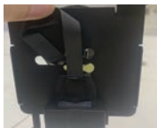
5. Place the cable plug in the wire slot.
