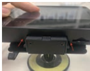
7. Align the display and insert into the stand.
